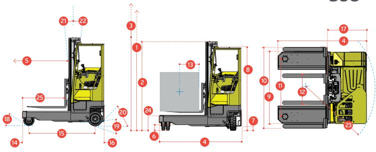
This compact truck features two rear wheel drive with rubber tyres and dynamic 360° 4 wheel steering rotation, contributing to faster procedures for manufacturing, distribution and logistics operations.
